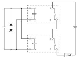
Note. The diode and zener diode are for the absorption of coil surge. (The coil does not have a polarity.) The opening/closing part does not have a polarity.
