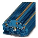
Test disconnect terminal block, nom. voltage: 1000 V, nominal current: 30 A, connection method: Push-in connection, Rated cross section:  $6~\text{mm}^2$ , cross section:  $0.5~\text{mm}^2$  -  $6~\text{mm}^2$ , color: blue
