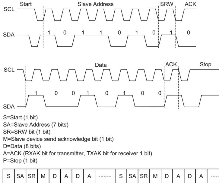
**I<sup>2</sup>C Communication Timing Diagram**
