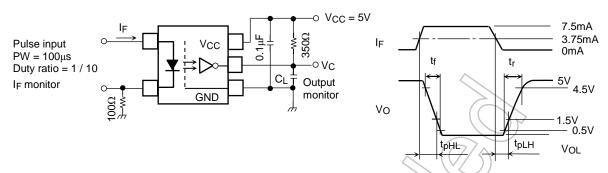
CL is approximately 15pF which includes probe and stray wiring capacitance.
