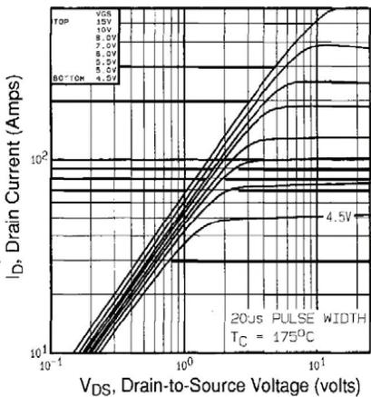
Fig. 2 - Typical Output Characteristics,  $T_C = 175\text{ }^\circ\text{C}$
